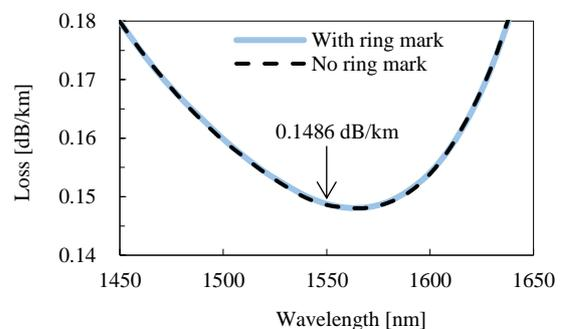
**Figure 5. Loss spectra of the fiber having  $A_{eff}$  of  $160 \mu\text{m}^2$  with and without ring mark.**
