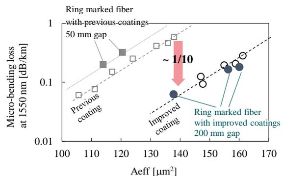
**Figure 4. Micro-bending loss as a function of  $A_{eff}$ .**
