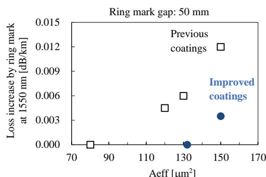
**Figure 2. Loss increase after placement of ring marks with a 50 mm gap.**
