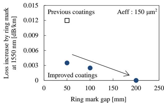
**Figure 3. Loss increase of a fiber with  $A_{eff}$  of  $150 \mu\text{m}^2$  as a function of ring mark gap.**
