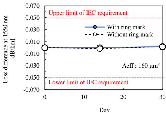
**Figure 7. Damp heat test result.**
