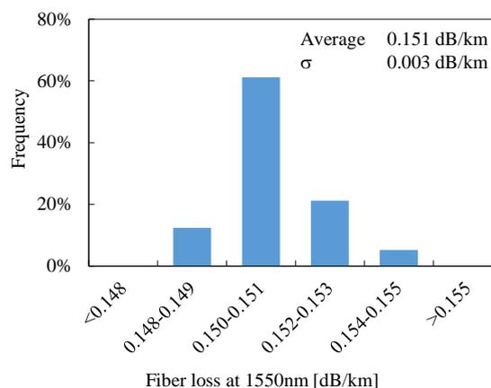
**Figure 6. Manufactured fiber loss distribution of ring marked fiber having Aeff of 150  $\mu\text{m}^2$ .**
