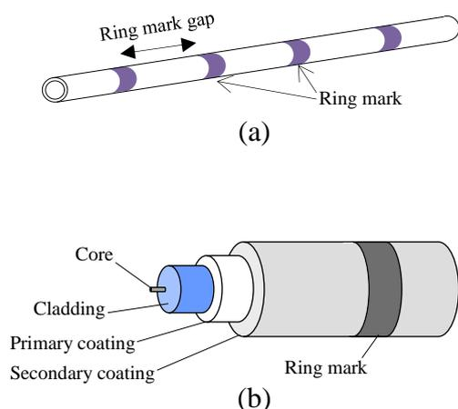
**Figure 1. Schematic drawing of ring marked fiber.**
