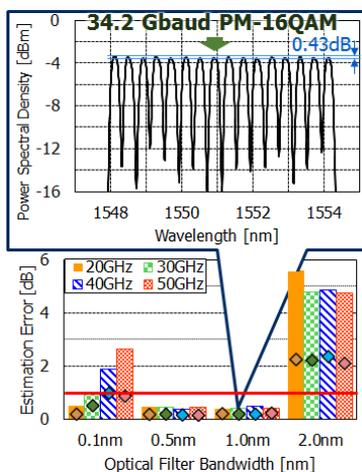
**Figure 7: Estimation error (Point: average, Bar: maximum) and optical spectrum with the monitor.**
