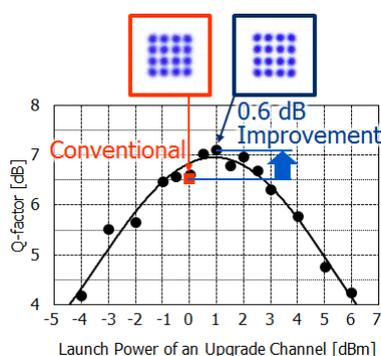
**Figure 8: Transmission performance over the PSCF loop.**
