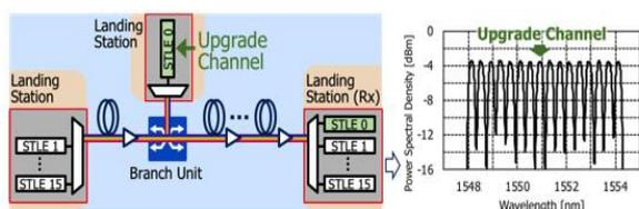
**Figure 1: A submarine cable system with a branch unit and the optical spectrum measured at Rx landing station.**
