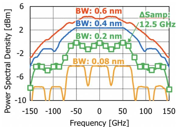
**Figure 2: Bandwidth dependency of the simple inline monitor in simulation.**
