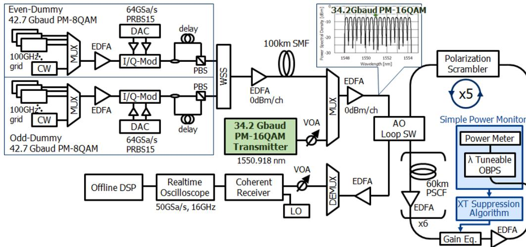
**Figure 6: Experimental setup for the demonstration of the proposed simple inline power monitor.**
