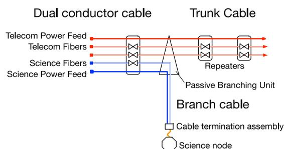
**Figure 3: Simplified diagram showing connection of a science observatory node to a commercial cable system.**
