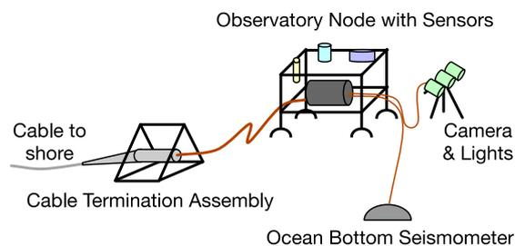
**Figure 1: Typical ocean observatory node showing connection of the CTA, node with junction box and external sensors.**
