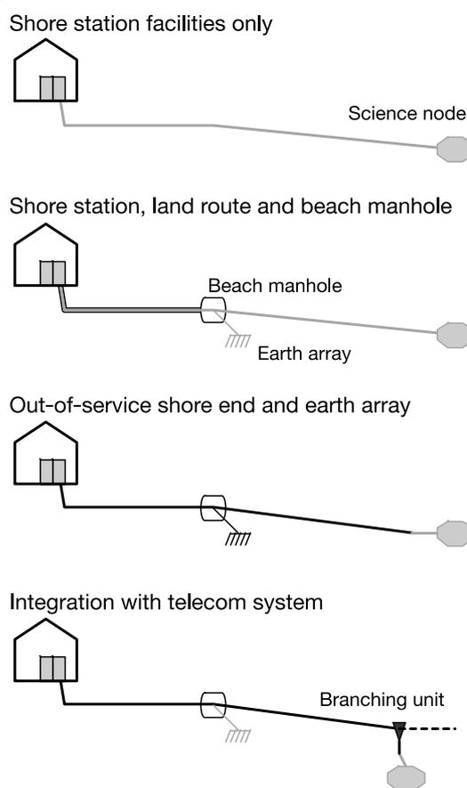
**Figure 2: Options for support of science observation showing shared infrastructure in black and infrastructure provided for science in grey.**
