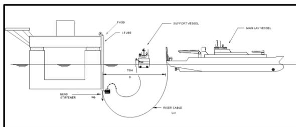
**Figure 1: Riser Installation Pull-in Prior to Lay Away**
