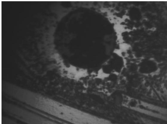
**Figure 3: Dirty Fiber Surface on a Dry Mate Connector**
