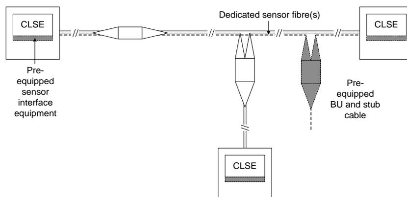
**Figure 1(c): Pre-Equipped Ocean Observation System components, shown in grey/dotted lines**
