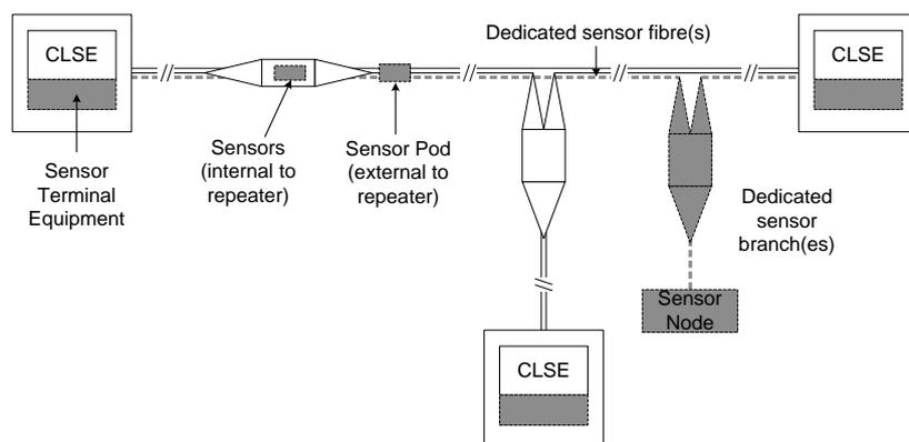
**Figure 1(b): Ocean Observation System components, shown in grey/dotted lines**
