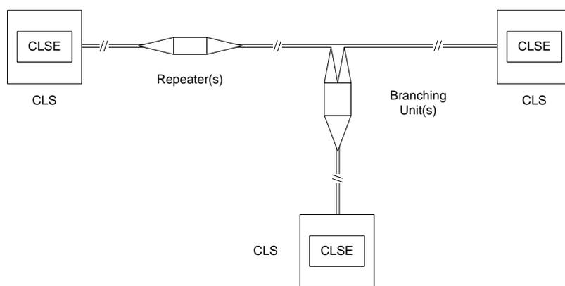
**Figure 1(a): Telecom System components**
