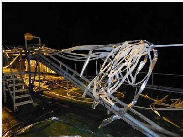
**Figure 5: Stripped Cable Waste Recovered with Coaxial Cable**
