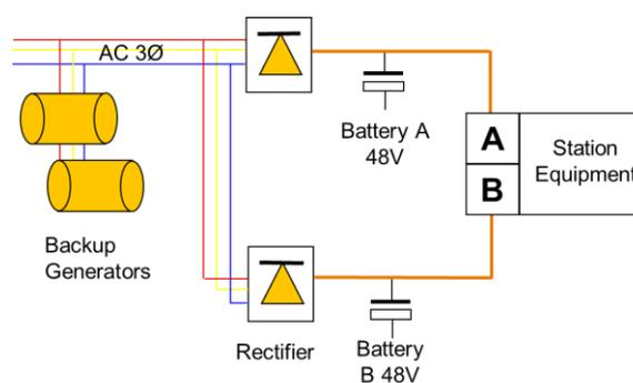
**Figure 1: Typical station powering**
