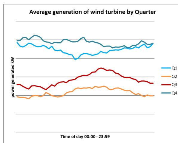
**Figure 5. Average generation profile throughout the day from a turbine closely located to the cable landing station**
