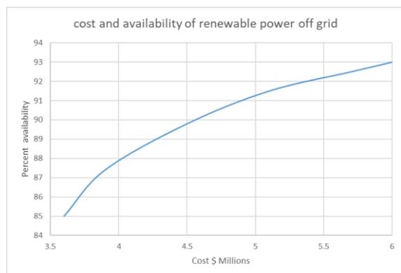
**Figure 6: Total cost of installed renewable generation and storage against % availability of renewable electricity.**
