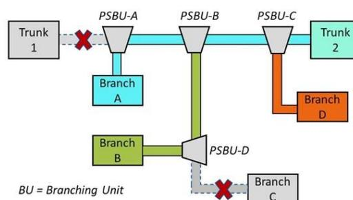
**(b) Powering Configuration after Cable Faults**
