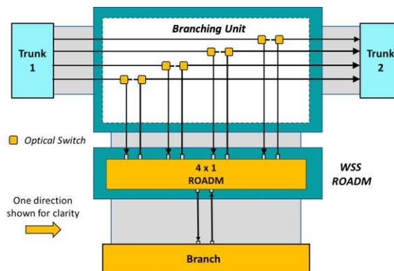
**Figure 8. BU/ROADM architecture with four trunk fiber pairs sharing ROADM spectrum access to one branch fiber pair**
