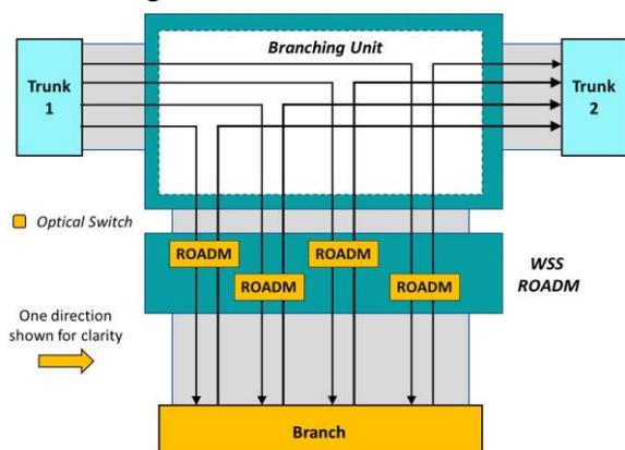
**Figure 4: BU/ROADM architecture with ROADM on every trunk fiber pair**
