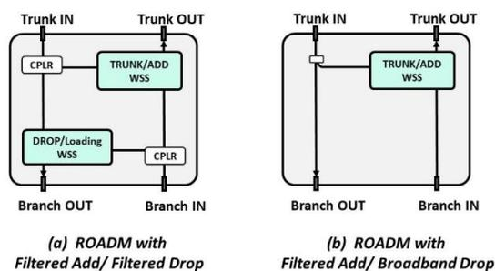
**Figure 1: High-level ROADM Filter Diagram**
