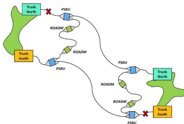
**Figure 9: Network with Cross-Cable interconnects**
