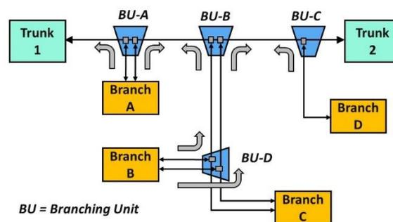
**Figure 2: Example of undersea network branch connectivity**
