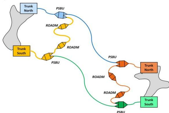
**Figure 11: Powering example for interconnected cables**
