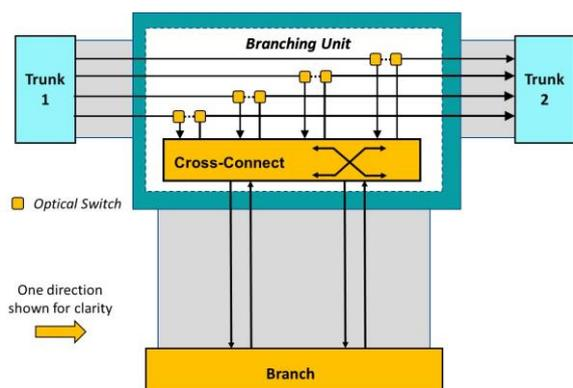
**Figure 7. BU architecture with flexible full fiber pair routing between trunk and branch**
