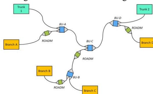
**Figure 3: Physical network routing between Branching Units**
