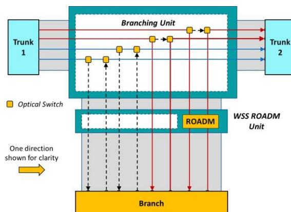
**Figure 6. BU/ROADM architecture with bypass switching on all fiber pairs, but ROADM on only one fiber pair**
