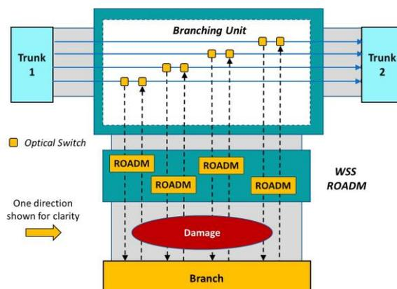
**Figure 5. BU/ROADM architecture with bypass switching for branch fault protection**
